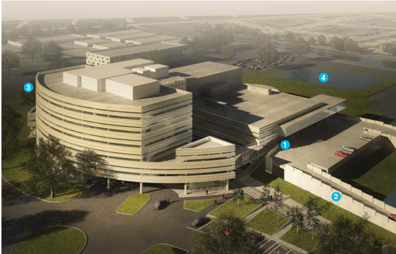
1. Critical functions are located at or above the second level to avoid damage during a flood event. 2. The emergency department ramp can double as a boat ramp during a flood. 3. The diesel fuel tank is raised in order to protect it from flood damage. 4. Detention ponds retain water during a storm event.
